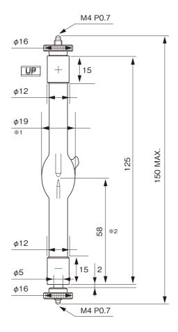
%1 Diameter excludes height of protuberance on lamp bulb. %2 Length to the center of the cold arc gap
